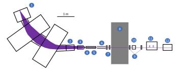
FIG. 1. Schematic of BGS + FIONA with the labels indicating the positions of 1. BGS, 2. BGS focal plane detector, 3. gas catcher, 4. RFQ, 5. RFQ trap, 6. acceleration region, 7. focusing element, horizontal and vertical steerers, 8. shielding wall, 9. focusing element, horizontal and vertical steerers, 10. C2 detector, 11. trochoid spectrometer, and 12. FIONA focal-plane detector. The purple shaded area or line represents the beam image of <sup>288</sup>Mc traveling through the BGS and FIONA.
