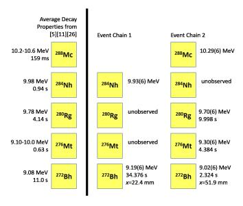
FIG. 4. (left) Average of known decay properties assigned to  $^{288}$ Mc and its daughters [5,11,29]; (right) details of decay chains detected at the FIONA focal plane. Unobserved decays within each decay chain are indicated as "unobserved" and are assumed to have been emitted out of the open end of the detector array. The x position of decays observed in the focal-plane detector is also given.
