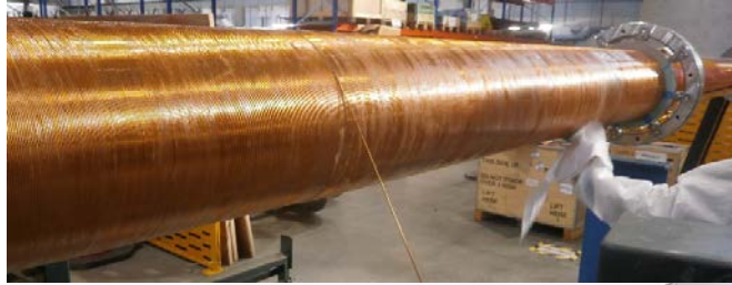
Solenoid coil being wound. Now complete.
